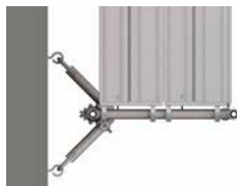
Figura 25: Support en V, configuration de base.
